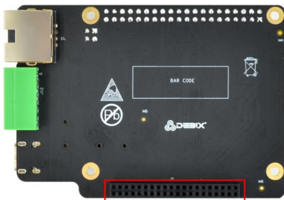
Figure 14 Female header of DEBIX I/O Board
