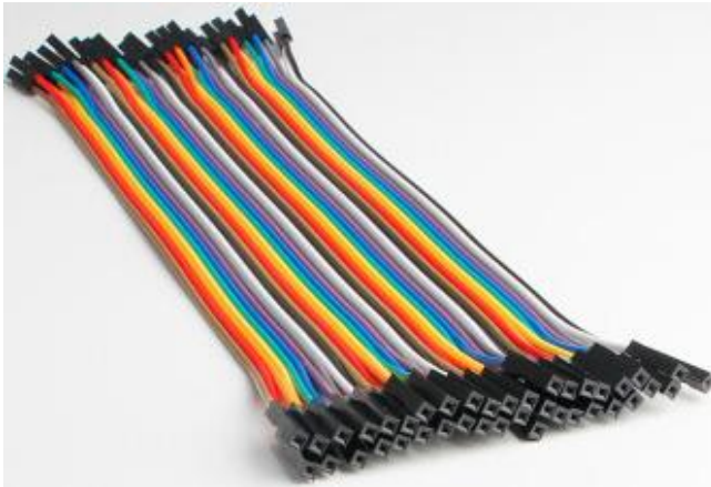
Figure 37 Female-to-female DuPont cables
